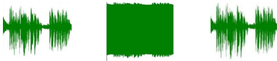
Fig 8: Original signal (Left), signal after Level 2 encryption (Middle) and Recovered file with high SNR (Right)
